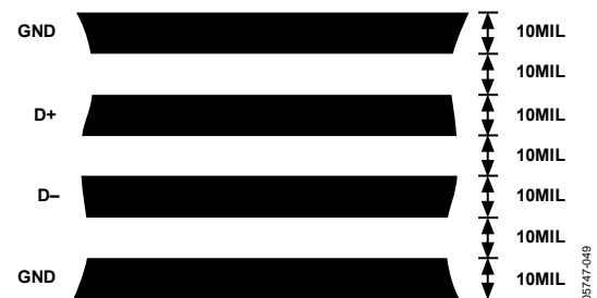
Figure 37. Arrangement of Signal Tracks
